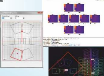
Aero OTS is our new innovative multi sensor Oblique Thermal System (OTS). Up to 9 thermal cameras based on Flir industrial OEM sensors are joint to a complex and ultra-high resolution system. Five sensors enable a contineous cross-track resolution of 3,200 pixels. Two front sensors and two back sensors deliver interesting oblique data e.g. to monitor facades of urban structures.
